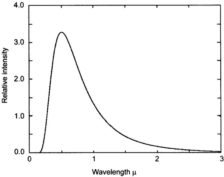
Figure 1.1.3.1 Variation of the relative intensity of black body radiation with wavelength ( $\mu$ ) at temperature 5700 °K, peaking at a wavelength of 0.5  $\mu$  in the visible region (Solar radiation)
