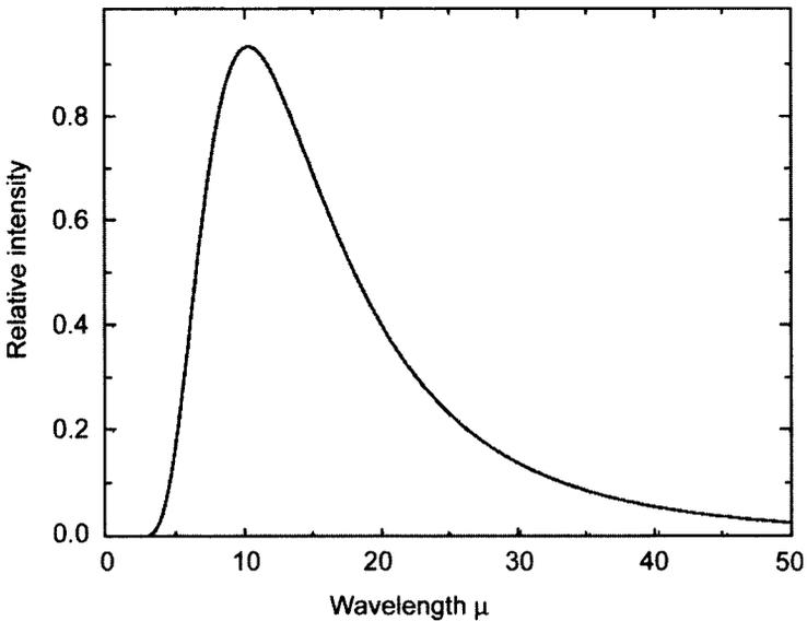
Figure 1.1.3.2 Variation of the relative intensity of black body radiation with wavelength ( $\mu$ ) at temperature 283 °K, peaking at a wavelength of 10  $\mu$  in the infra-red region (Terrestrial radiation)
